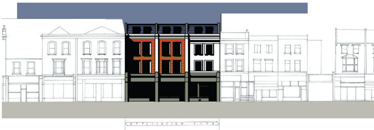
Tottenham High Road Frontage (Note 1 st & 2 nd Floors set back behind side to No 704, 3 rd floor set back further)
